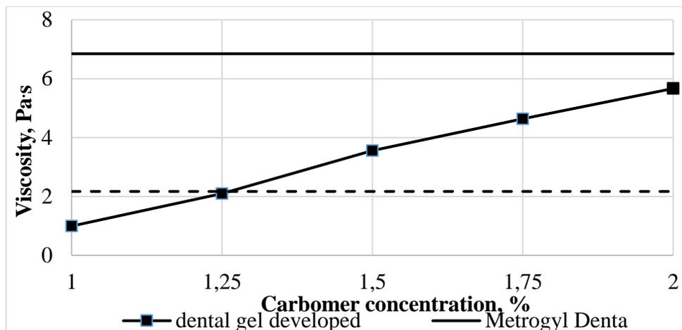
Fig. 2. The dependence of the structural viscosity of the dental gel at a shear rate of  $41.6 \text{ s}^{-1}$  on the concentration of carbomer in comparison with reference drugs (at  $25 \text{ }^\circ\text{C}$ )
