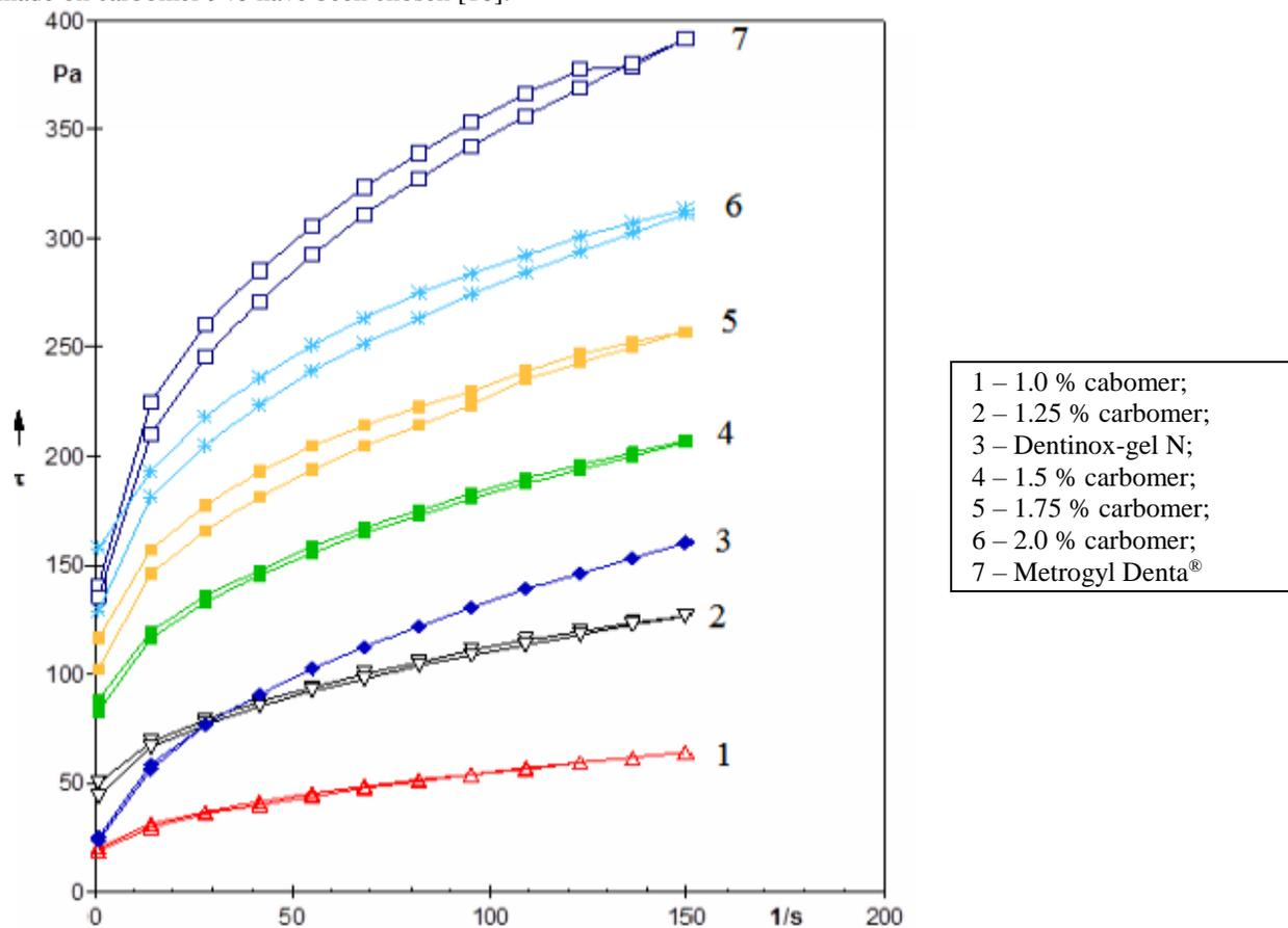
Fig. 1. Rheograms of dental gel, depending on the concentration of carbomer in comparison with reference preparations (at 25 °C)
