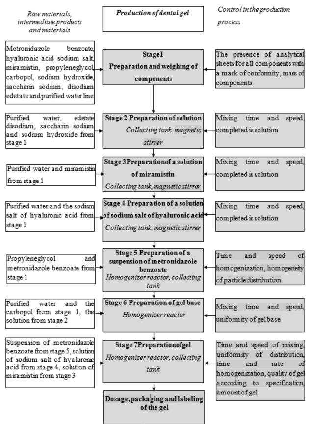
Fig. 1 . Flow chart of production of combined dental gel
